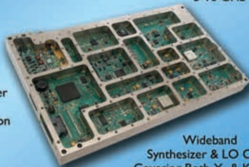
Amplified Switch Filter Bank 9 Selectable Bands 5-18 GHz
